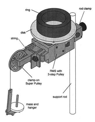
Fig. 1. Rotational inertia setup of disk and ring
